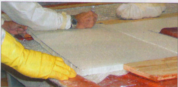
H8PP is the designation of one of several polypropylene structural boneycomb cores developed by Nida-Core for fabricating lightweight panels and parts.
